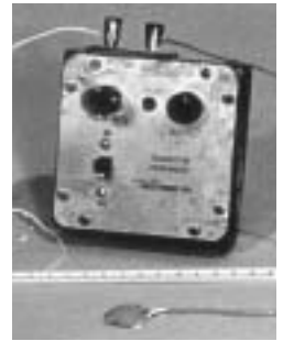
The first wearable, transistorized, battery-powered pacemaker, above, was developed in 1957 by Earl Bakken, middle. The Chardack-Greatbatch pacemaker, below, is a later-generation implantable device.
